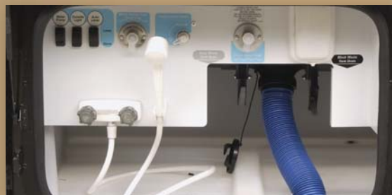
EXTERIOR SERVICE CENTER Large, color-coded labels make hookups a snap. The QuickPort® service connection hatch allows the bay doors to close when hookups are connected.
