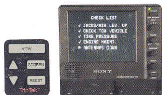
▲ The available TripTek™ computer displays trip information on the rearview monitor, including: distance to scheduled destination, time to destination, distance traveled, time traveled, fuel economy and a handy pre-trip checklist.
