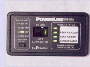
The Powerline™ Energy Management System allows two roof air conditioners to operate on 30 amps of available power.
