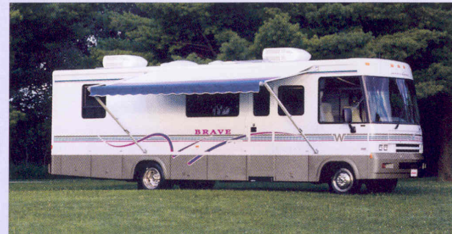
F32T The Brave's newly designed awning rail with built-in gutter keeps things dry by channeling water away from the awning.
