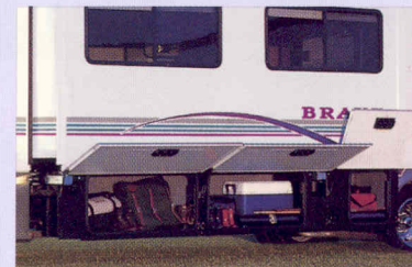
F35C The StoreMore Hydraulic Slideout System features exterior storage compartments that extend with the room to make loading and unloading easier.
