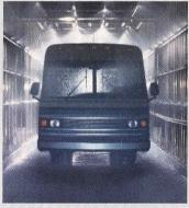
To simulate the ferocity of a thunderstorm, each Winnebago motor home is subjected to an exterior water leak test in this tunnel filled with highpressure spray nozzles.
