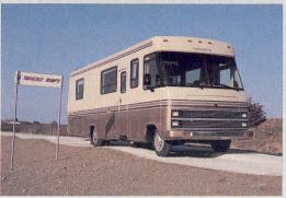
Winnebago Industries' test track is one-of-a-kind in the motor home industry. In a half mile of the track, a motor home encounters two-inch-high cobble stones, a high-crowned intersection, 3r-inch chatter bumps, four-inch chuck holes, two-inch sine wave bumps and staggered six-inch high bumps. The track also tests the reliability of motor homes' brakes on 20 and 30 percent grades.
