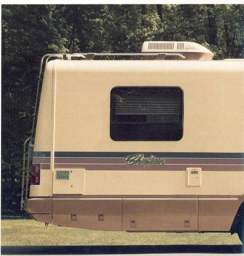
The storage bays are wide and roomy and the two deep-cycle batteries pull out of a separate storage compartment for easy access. An extra deep rear storage bay will accommodate longer items like skis or golf clubs.
