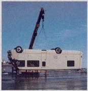
To really put motor homes to a test. Winnebago Industries drops them on their tops. Doors must still open and close easily. Appliances and cabinets must stay firmly in place. The motor home must prove to be structurally sound in order to pass the
