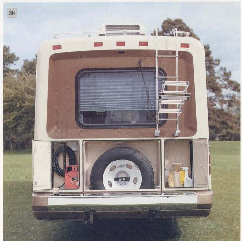
separate insulated inner rear wall. **38.** The unique rear cap has three compartments not found on most other motor homes: one for your own odds and ends; one for the spare tire; and a lighted compartment with stand-up access to the electrical cord, cable TV hookup and optional garden hose/reel.
