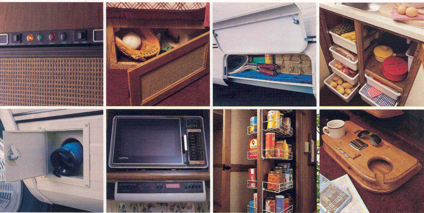
Top row L to R: Eye-level refrigerator controls; dinette storage; dual-locking exterior storage; drawers under sink. Bottom row: Sewer hose compartment; microwave oven and monitor panel; roll-out pantry; oak beverage tray.
