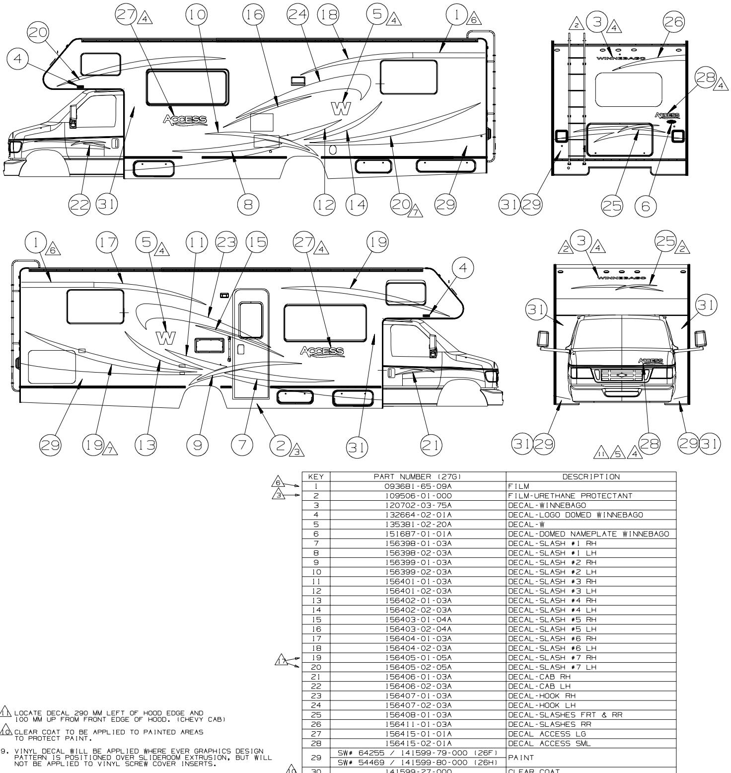
LOCATE DECAL 290 MM LEFT OF HOOD EDGE AND 100 MM UP FROM FRONT EDGE OF HOOD. (CHEVY CAB)
