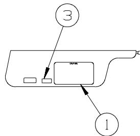
LABELS SHALL BE LOCATED ON OPPOSITE SIDE OF VISOR THAT THE AIR BAG LABEL IS INSTALLED ON.
