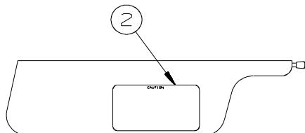
LABELS SHALL BE LOCATED ON OPPOSITE SIDE OF VISOR THAT THE AIR BAG LABEL IS INSTALLED ON
