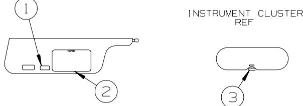
LABELS SHALL BE LOCATED ON OPPOSITE SIDE OF VISOR THAT THE AIR BAG LABEL IS INSTALLED ON
