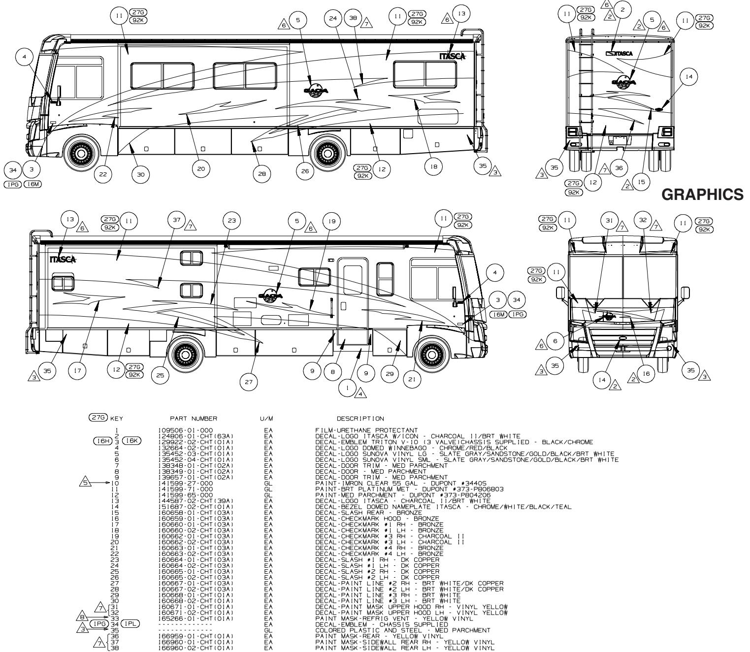
USE PAINT MASK ON REFRIGERATOR VENT ON STANDARD GRAPHICS WHEN PAINT IS APPLIED TO VENT.
