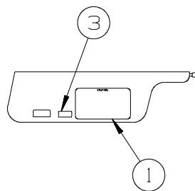
LABELS SHALL BE LOCATED ON OPPOSITE SIDE OF VISOR THAT THE AIR BAG LABEL IS INSTALLED ON.
