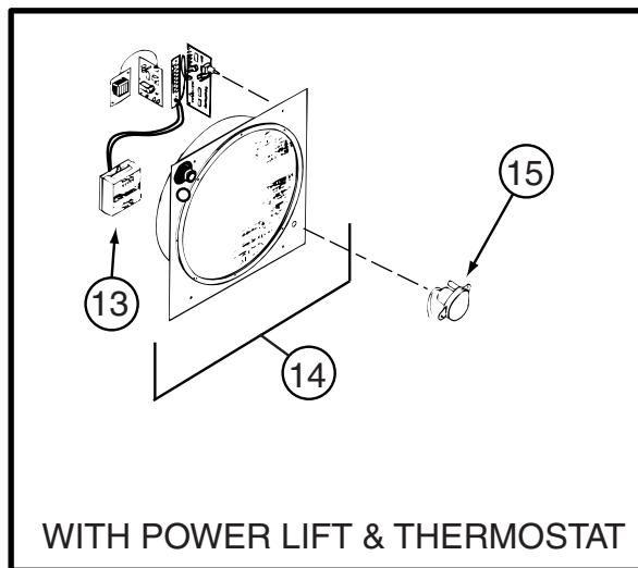
**COMPONENT PARTS FOR WINDOW & VENT LAYOUT**
