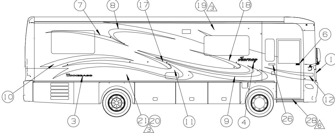
DIE CUT ACRYLIC 3M FILM USED TO PROTECT FULL BODY PAINTED UNITS.
