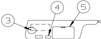
LABELS SHALL BE LOCATED ON OPPOSITE SIDE OF VISOR THAT THE AIR BAG LABEL IS INSTALLED ON
