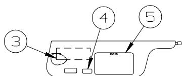
LABELS SHALL BE LOCATED ON OPPOSITE SIDE OF VISOR THAT THE AIR BAG LABEL IS INSTALLED ON
