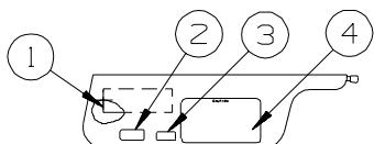
LABELS SHALL BE LOCATED ON OPPOSITE SIDE OF VISOR TAHT THE AIR BAG LABEL IS INSTALLED ON.
