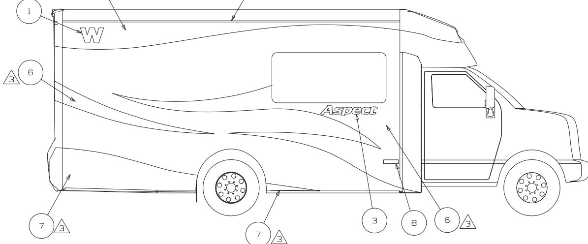
**5A** USE PROTECTIVE FILM 145487-02-000 TO COVER UNSEALED ROOF SEAMS.
