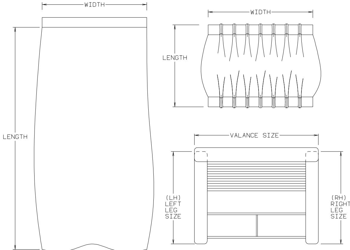
NOTE: USE THIS ILLUSTRATION WHEN DETERMINING LENGTH AND WIDTH MEASUREMENTS FOR CURTAINS. YOU WILL NOTE THE WIDTH MEASUREMENT IS TAKEN ON THE TOP OF THE CURTAIN WITH THE CURTAIN FULLY EXTENDED. THE LENGTH MEASUREMENT IS TAKEN FROM TOP TO BOTTOM. LEFT AND RIGHT WINDOW LEGS ARE DETERMINED WHEN FACING THE WINDOW.
