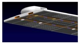
Are all ducts created equal? Not at all. With the exclusive TrueAir Maximum Comfort AC, we employ an advanced ductwork design that ensures consistent, precision airflow throughout the coach. The ductwork is formed, rather than routed, and possesses a unique D-shape with radiused edges that reduce drag and turbulence as conditioned air travels along the length of the coach (see ductwork graphic at left). And with multiple units all operating through a single ducting
