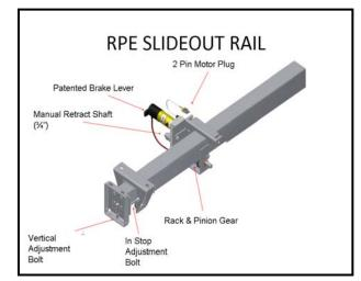
**Digi-Sync RPE** = Rack & Pinion / Electronic – This mechanism is Power Gear's variation of the original Kwikee® Digi-Sync 2-arm slide-out mechanism. A rack & pinion drive is employed versus the ACME screw drive. The synchronization process is controlled by a 'control' module or ECM.
