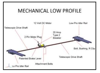
**RPM** = Rack & Pinion / Mechanically-Synchronized – This mechanism is a 2-arm installation that's powered by a single electric motor. The motor / gearbox assembly is positioned between the two arms and a 'drive shaft' powers / actuates both arms equally. A variation exists with one arm being a powered arm assembly and the second arm being a *driven* arm.
