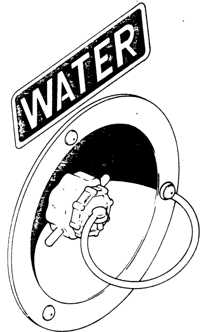
CITY WATER CONNECTION
