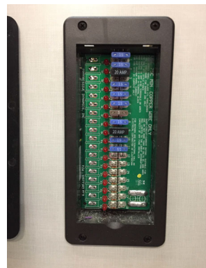
House 12-Volt Fuses -Typical View
