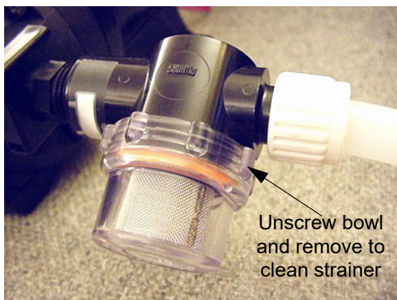
Water Pump Strainer -Typical View
