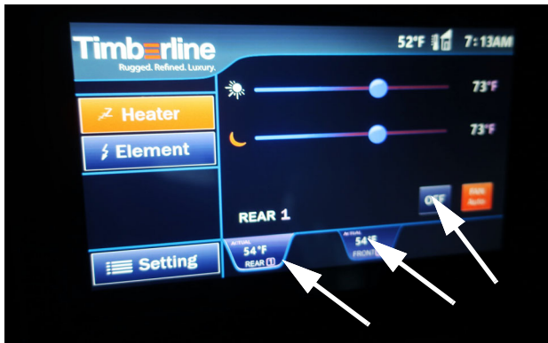
To have the hot water on with NO heat, select the Heater button and turn the available zones to OFF -Typical View
