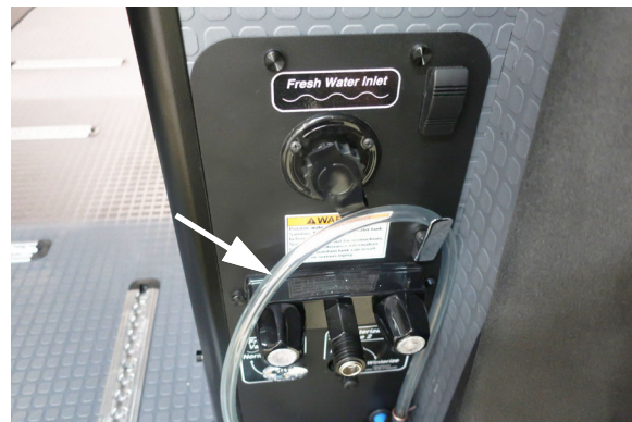
Use the siphon tube attached to the water center and place it in the chlorine solution container and turn the pump on to begin siphoning contents. (Typical View)
