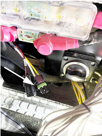
Location of AC Sense and ignition power connectors. -Typical View
