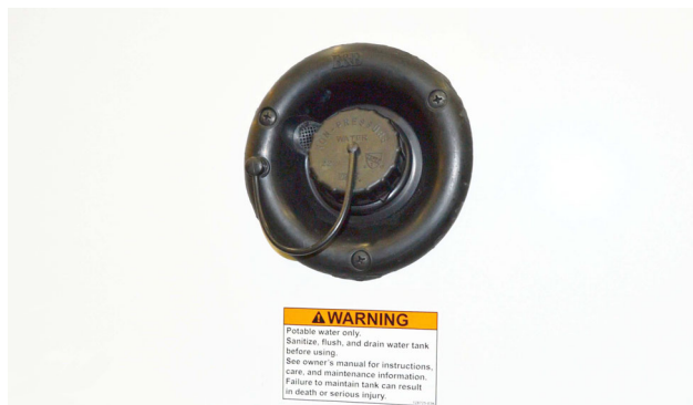
Water Tank Gravity Fill -Typical View
