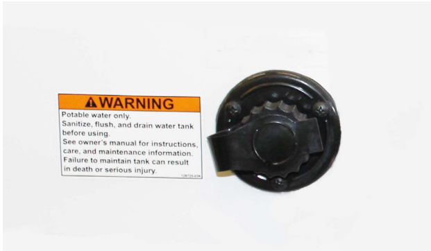
Fresh (City) Water Inlet -Typical View
