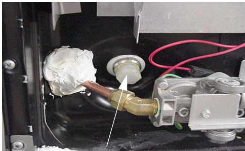
Water Heater Drain Plug (Remove with socket)
