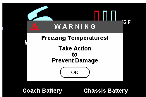
Freezing Temperature Warning Screen -Typical View
