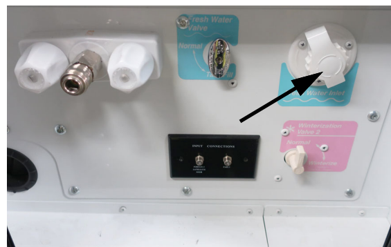
Fresh (City) Water Inlet (Located behind the drivers side Water Service Center door) -Typical View
