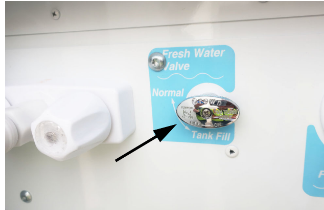
Fresh Water Valve in normal position (Located in water service center) -Typical View
