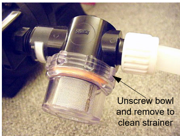
Water Pump Strainer -Typical View
