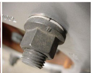
Steel Wheel Lug Nut and Washer (Hex Flange Nut with Split Cone Washer)
