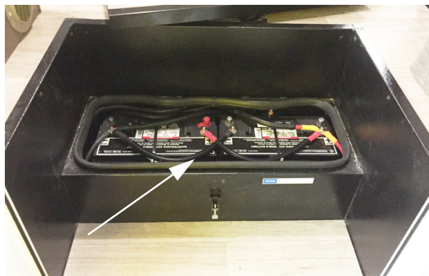
House Batteries (Entrance Step Removed) -Typical View
