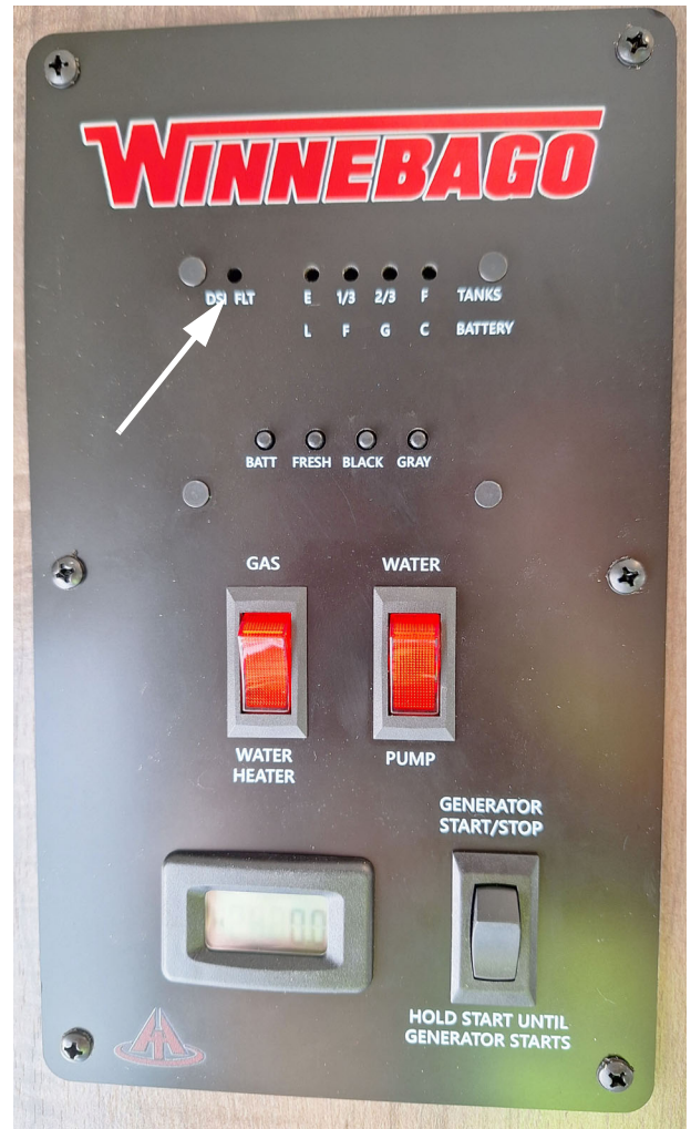
Pilot Out light (Located on the control panel) -Typical View
