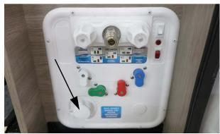
Tank Fill Inlet (Located behind the passenger rear door)
