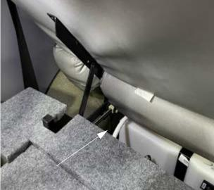
To access the water pump strainer, first put the sofa in between the full couch position and the full bed position
