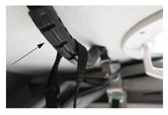
5. Press up firmly on the handles and lift Pop-Top up until shocks take over and extend Pop-Top to the extended position shown below.
