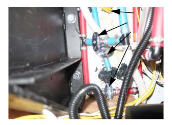
Waterlines and Tank Drain Valves
