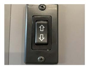
2. Push up arrow to raise the bed into a couch or the down arrow to lower the couch into a bed.
