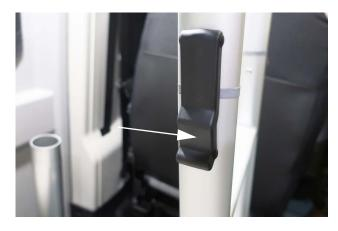
8. Attach the ladder to the Driver's side ladder clamps provided to hold the ladder in place.
