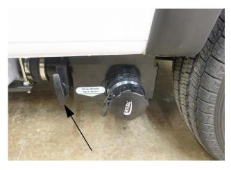
5. Rinse sewage drain hose thoroughly with water before stowing.
