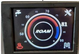
• **Hot Water Icon**, the system will cycle and maintain the hot water heat exchanger so that hot water is available on demand.
