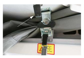
3. Pull turn knob out and twist to the left until the latch is extended.
