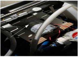
The water pump strainer is located to the left side near the wheel well
