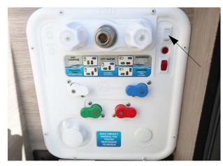
Water pump switch location on Water Center Panel -Typical View
