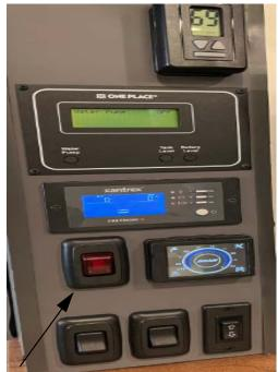
DO NOT operate the holding tank heater unless you are providing a supplemental 12-volt power source to recharge the house batteries. This means either the shoreline cord must be plugged into a 120-volt source, the auxiliary generator must be operating, or the chassis engine must be running (such as when driving down the road). This will prevent excessive discharge of the house battery.
