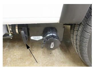
Gray waste tank drain valve (shown closed- pull lever out to drain)
