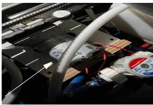
Water Pump Accessible when the couch is stopped halfway through transition into sofa
