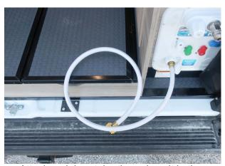
Attach a siphon tube then place it in the chlorine solution container and turn the pump on to begin siphoning contents.
