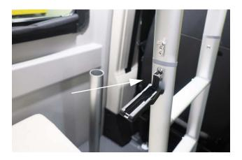
7. Attach the 2 latches and lock them down to lock the 2 halves of the ladder in place.
