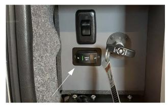
House/Coach Battery Disconnect switch (Located near sliding door)
