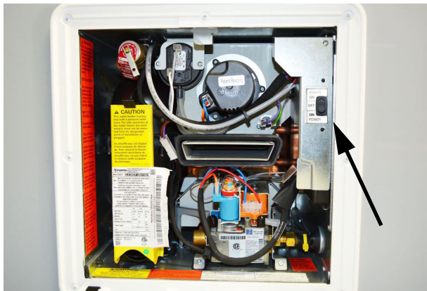
Water Heater Power Switch (Located behind water heater access panel on exterior of the motorhome) -Typical View
