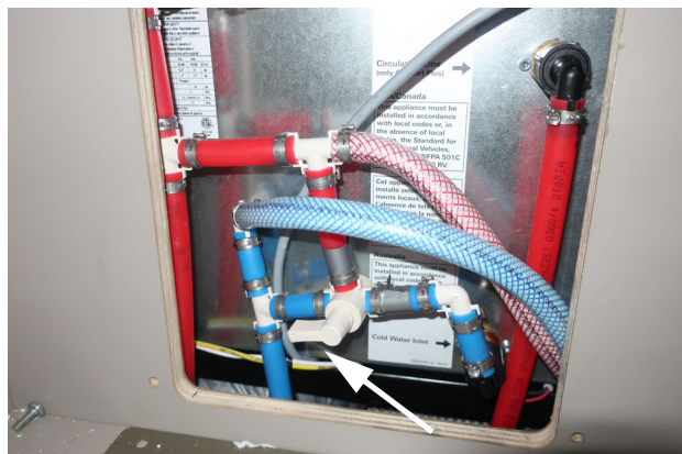
Winterization Valve #1 Water Heater Bypass on model 524R located inside the galley. (Shown in Normal position). -Typical View
