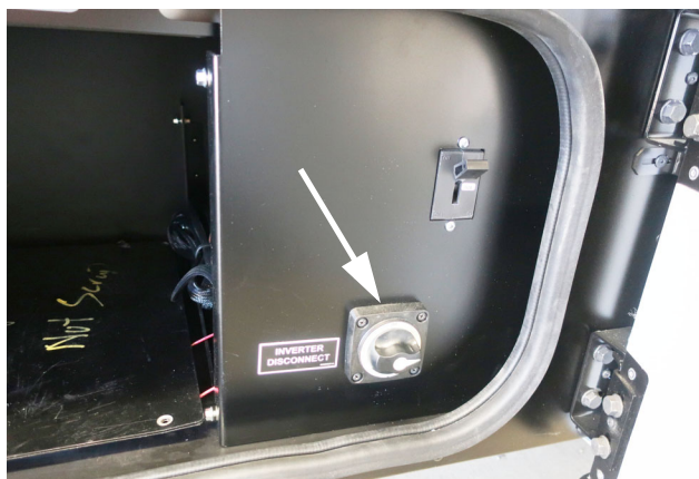
Inverter/charger disconnect switch. (Located in the passenger side compartment) (Options 52D 78G shown) -Typical view
