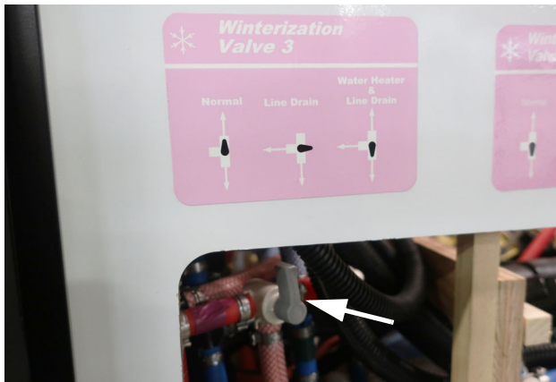
Winterization Valve #3 Located in the gear garage behind the removable panel on the 524T. (Shown in the normal position). -Typical View
