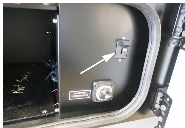
250 Amp Circuit Breaker (Located in the passenger side compartment) (Options 52D 78G shown) -Typical view
