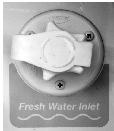
Fresh (City) Water Connection “Fresh Water Inlet” (Located on the driver's side sidewall) -Typical View
