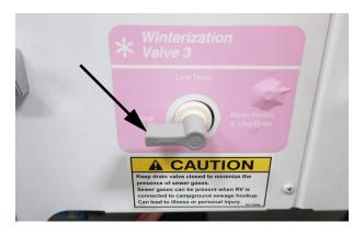
Place the Winterization Valve 3 into the "Normal" position.
