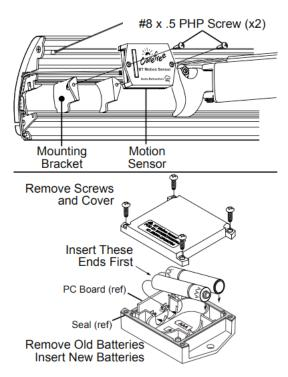
Awning motion sensor battery replacement (see below for details).
