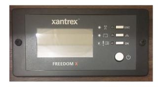
When the inverter/charger is not being used, it should be shut off at the charger panel. The inverter/charger could drain the house batteries if the shoreline is not connected to external power and the inverter/charger disconnect switch is on.
