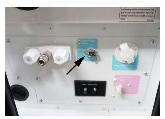
Fresh Water Valve (Drain). (Shown in the closed position). -Typical View
