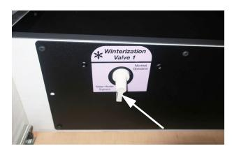
Place the Winterization Valve 1 in the "Water Heater Bypass" position.
