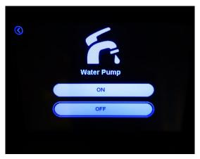
Select the Water Pump icon on the main menu to access the water pump ON/OFF button. -Typical View
