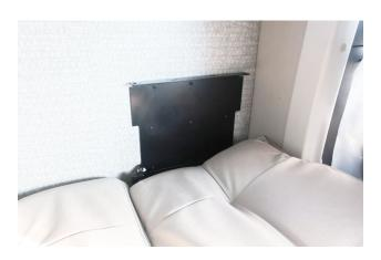
5. Located in the infocase is a magnetic panel that is placed on the table in the down configuration. This protects anything from making contact with the hard metal of the table anchor.
