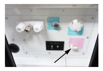
Winterization Valve #2 in "Winterize" configuration (Panel located inside the Water Service Center on the drivers side).
