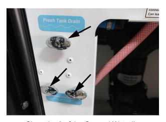
Close the 3 of the General Waterline drain valves located at the Water Service Center (Shown in the closed position).
