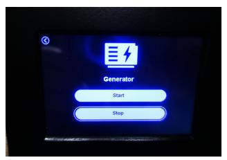
Select the Generator Icon on the main menu to access the Generator start/stop screen.
