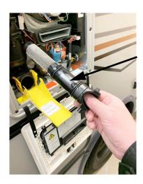
Water inlet strainer pulled out and removed.
