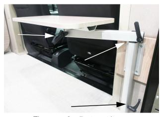
There are 3 adjustment levers that alter the height, length, and position of the table.
