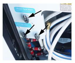
Open 3 of the General Waterline drain valves located at the Water Service Center (Shown in the open position).
