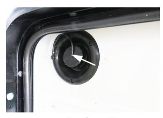
Water Tank Gravity Fill
