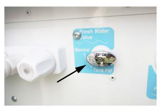
Fresh Water Valve in normal position (Located in water service center)
