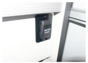
Water Pump Switch in the rear of the galley.
