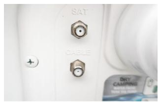
Satellite Dish and Cable TV Connections (Located on the Water Center Panel)
