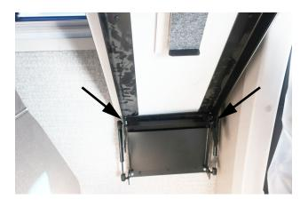
2. The table will then swing down flush with the seat-remove cushion to avoid pinching fabric.
