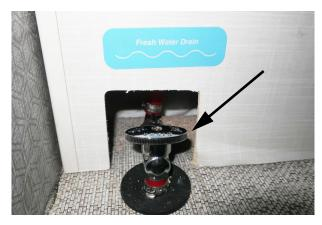
Close the 1 General Waterline drain-Passenger Side Compartment Drain Valve (Shown in the closed position). -Typical View
