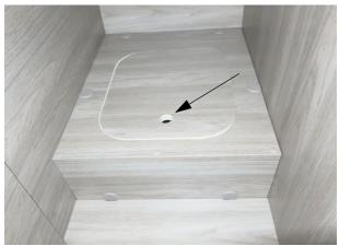
To access the water pump strainer, first locate the hole in the passenger side bed lower forward storage area.
