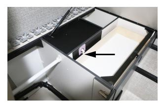
Lift the passenger's side bed to reveal Winterization Valve #1.
