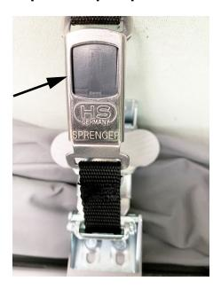
Locate the retention clamps on the driver's and passenger's side of the Pop-Top, and push the black button to release.
