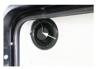
Water Tank Gravity Fill
