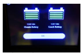
Select the Coach battery icon on the main menu to view the level of charge (voltage) of the Chassis battery and the Coach Battery. -Typical View
