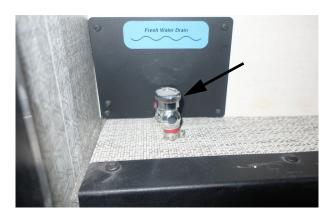
Open and drain the one General Waterline Drain- Passenger Compartment Drain Valve (Shown in the open position). -Typical View
