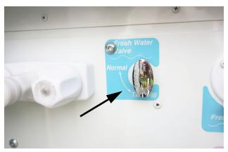
Fresh Water Valve in tank fill position (Located in water service center)
