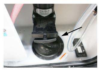
Sewage Drain Outlet with drain valve (Located inside the Water Service Center on the drivers side pull valve outward to open)
