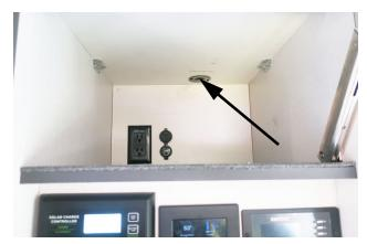
Roof Access Port (Located inside rear overhead cabinet). -Typical View
