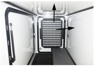
The hidden support brackets are located on the wall and the ceiling in the Gear Garage. (Use a magnet to locate.)
