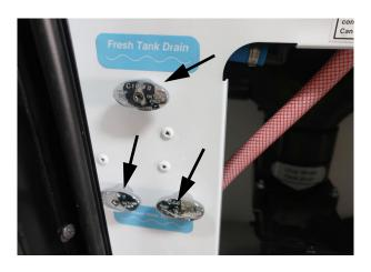
3 of the General Waterline Drain Valves. (Shown in the closed position) -Typical View
