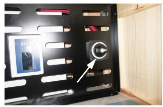
Inverter/charger disconnect switch. (Located inside the passenger's side compartment door next to the inverter).
