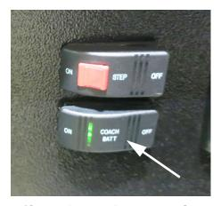
House/Coach Battery Disconnect Switch (Located near entrance door or end of galley, depending on model)
