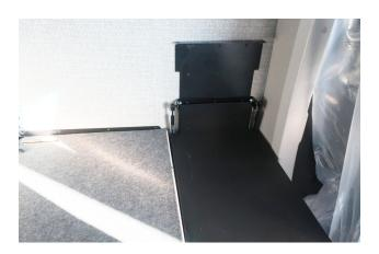
3. Extend the table block out to lock the table in the extended position.
