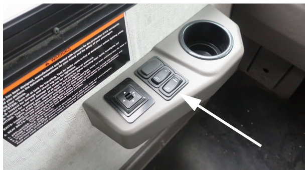
Mirror Heat Switch (Located on driver side trim panel) -Typical View
