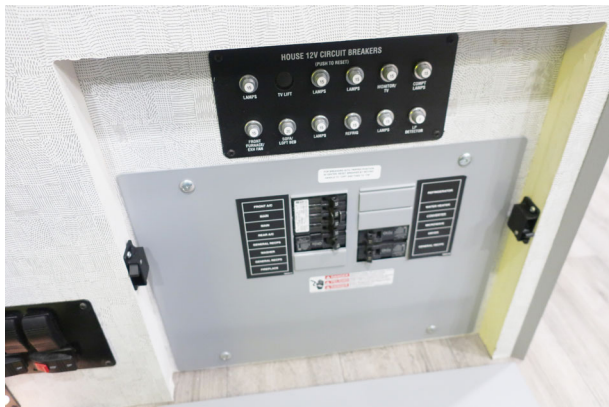
House 12-Volt Circuit Breakers -Typical View
