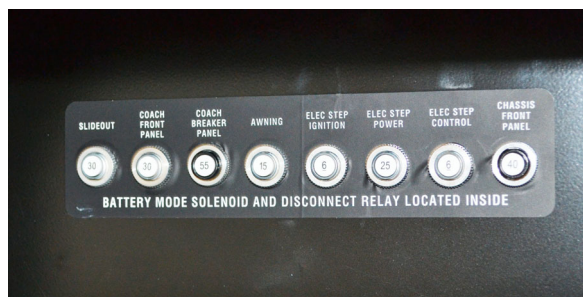
Automotive Chassis and House 12-Volt Circuit Breakers (Located inside passenger compartment) -Typical View
