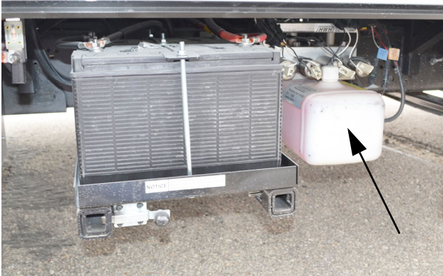
Hydraulic Oil Reservoir (Located in mid-passenger side compartment) -Typical View
