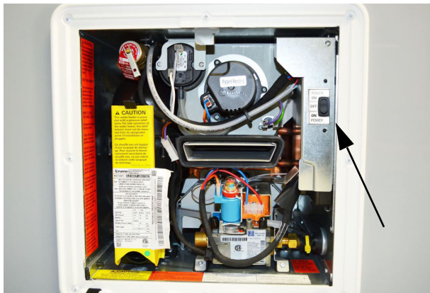
Water Heater Power Switch (Located behind water heater access panel on exterior of the motorhome)
