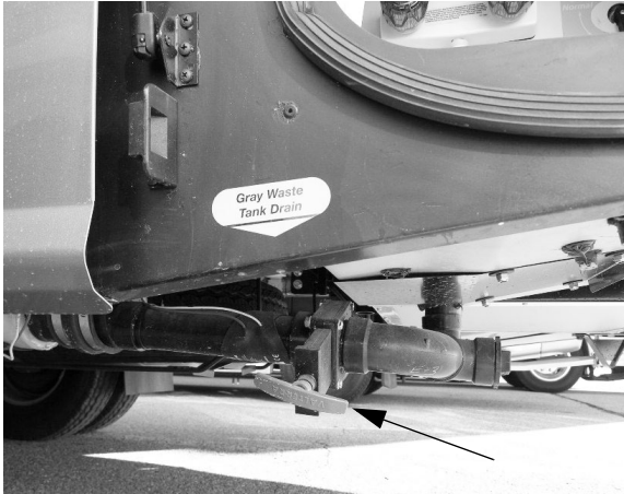
Gray Waste Tank Drain Valve (Located beneath rear driver side of the motorhome) -Typical View
