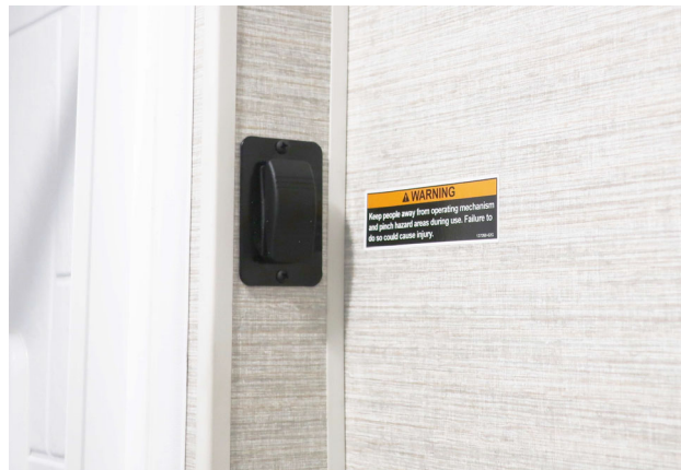
Murphy Bed Switch (Located near shower)
