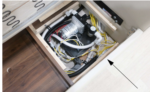
Water Pump (Located beneath sofa seat) -Model 24D shown
