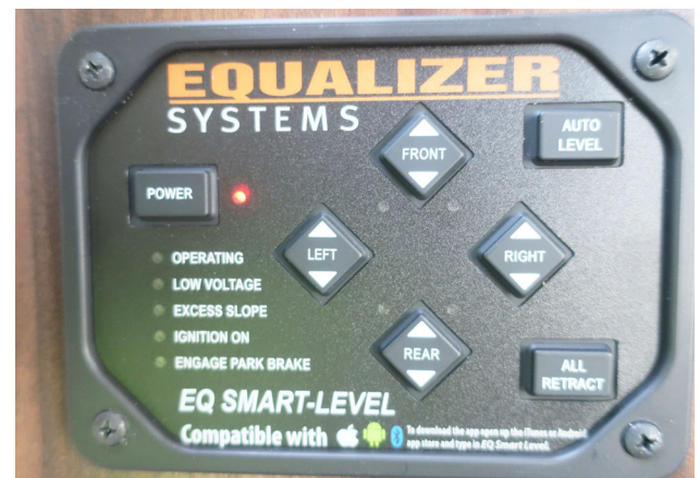
Equalizer Control Panel -Typical View
