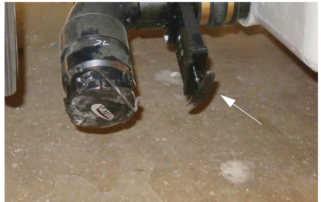
Black Waste Tank Drain Valve (Located in driver side compartment) -Typical View
