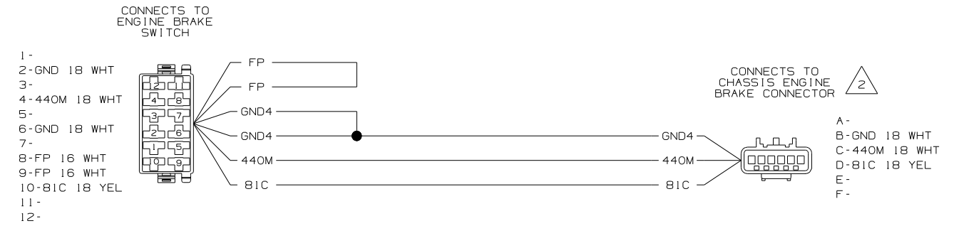
WIRING DIAGRAM-ENGINE BRAKE SWITCH (WIRE ASM 157534-02 REV-E)
