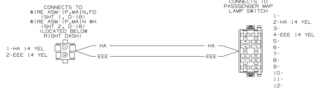
WIRING DIAGRAM-SIDEWALL,FRONT (WIRE ASM 149199-03 REV-F)
