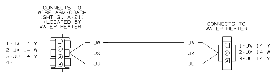
WIRING DIAGRAM-JUMPER WTR HTR (WIRE ASM 142263 REV-A)
