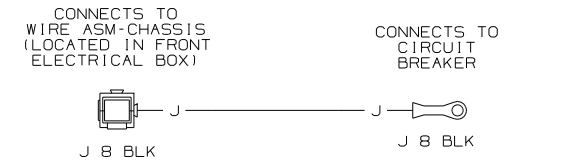
WIRING DIAGRAM-CRT BRK,POWER (WIRE ASM 103991-01 REV-G)
