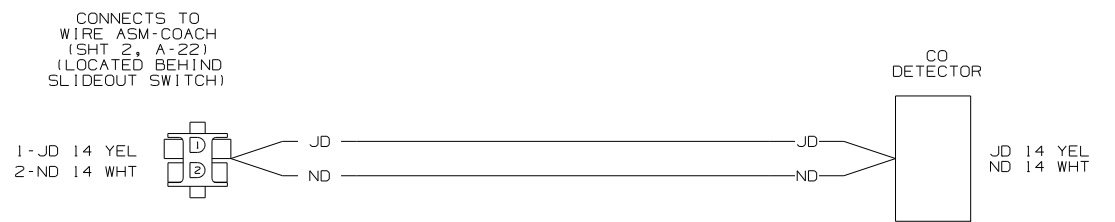
WIRING DIAGRAM-EXTENSION, 2-PIN (WIRE ASM 149130 REV-C)
