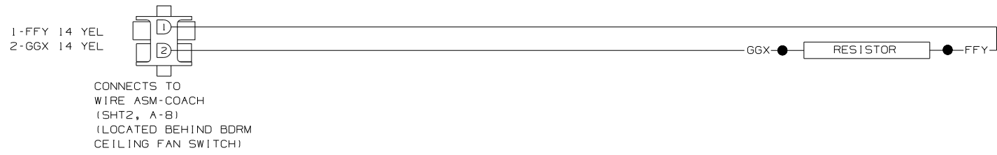
WIRING DIAGRAM-RESISTOR, FAN (WIRE ASM 140195 REV-A)
