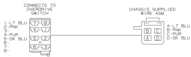
WIRING DIAGRAM-OVERDRIVE SWITCH (WIRE ASM 137626-01-000 REV.E) (WORKHORSE 20,700#-19.5 TIRE)
