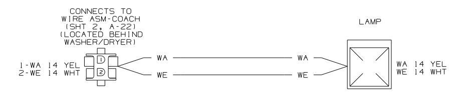
WIRING DIAGRAM-SIDEWALL,LEFT (WIRE ASM 77093-15 REV-AG)
