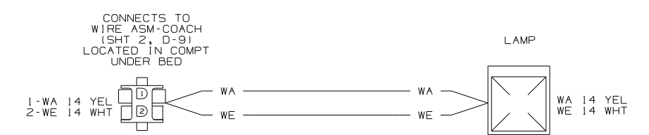
WIRING DIAGRAM-EXTENSION (WIRE ASM 149130-01 REV-B)
