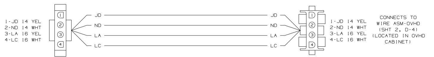
CONNECTS TO WIRE ASM-CHASSIS (SHT 1, D-8) (LOCATED UNDER STOVE CABINET) 1-JD 14 YEL 2-ND 14 WHT 3-LA 16 YEL 4-LC 16 WHT WIRING DIAGRAM-SLIDEOUT, ROOM (WIRE ASM 142435 REV-C)
