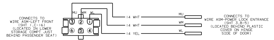
WIRING DIAGRAM-SIDEWALL (WIRE ASM 135846-01) 222HD & 222FD ONLY
