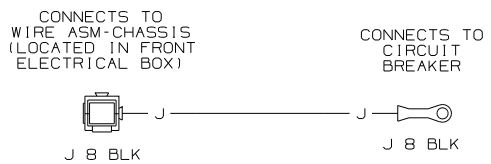
WIRING DIAGRAM-CRT BRK,POWER (WIRE ASM 103991-01 REV-G)
