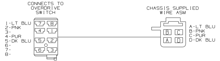
WIRING DIAGRAM-OVERDRIVE SWITCH (WIRE ASM 137626-01-000 REV.E) (WORKHORSE 20,700#-19.5 TIRE)
