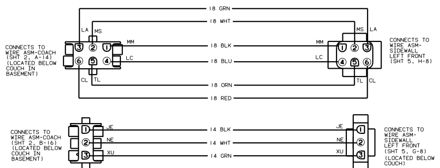
① WIRING DIAGRAM-EXTENSION, SLIDEOUT (WIRE ASM 115818-02)
