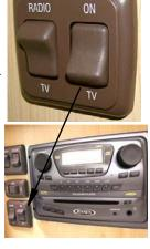
the TV is not in use, the Master Power switch should be turned off to eliminate drain on the 12-volt house battery.
