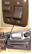
in use, the Master Power switch should be turned off to eliminate drain on the 12-Volt house battery.
