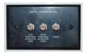
Satellite Dish and Cable TV Connections (Located in utility compartment, shoreline compartment, or water service center, depending on model)
