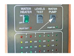
NOTE: Some models may be equipped with a Water Pump switch in the water service center on the outside of the motorhome or within the bathroom area for your convenience.
