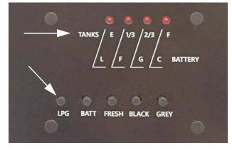
The propane level is registered by a sending unit on the tank. The gauge mounted on the side of the tank will give a more accurate indication of actual tank level if needed.
