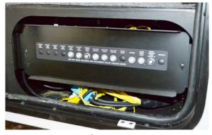
Automotive Chassis and House 12-Volt Circuit Breakers (Located inside passenger compartment) -Typical View
