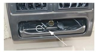
Bluetooth Microphone (Located on lower dash) -Typical View (if equipped)
