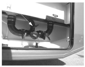
Black Waste Tank Drain Valve #2 (Front)
