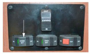
Chassis Battery Disconnect Switch (Located near entrance door)
