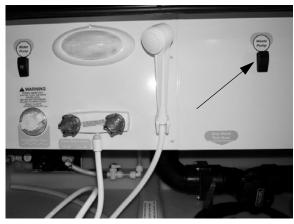
Waste Pump Switch (Located in water service center)
