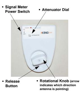
Digital Antenna Signal Meter (Located on ceiling)
