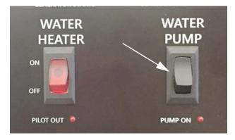
NOTE: Some models may be equipped with a Water Pump switch in the water service center on the outside of the motorhome or within the bathroom area for your convenience.
