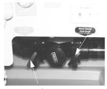
1st - Pull Black Waste Tank Drain Valve to drain Black Water (sewage) Tank, then close.
