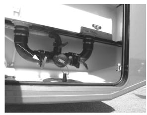
Gray Waste Tank Drain Valve (Located in water service center)
