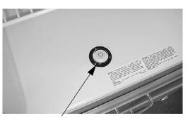
Place bubble level in bottom of refrigerator
