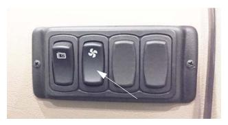
Defrost Fan Switch (Located on dash) -Typical View
