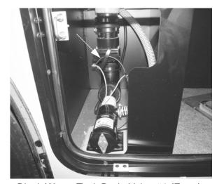
Black Waste Tank Drain Valve #1 (Front)
