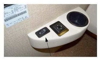
Mirror Heat Switch (Located on driver side trim panel) -Typical View
