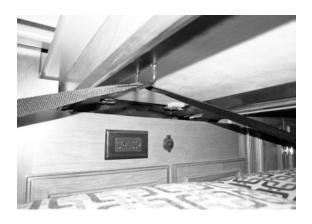
3. Latch strap and tighten as necessary for security.
