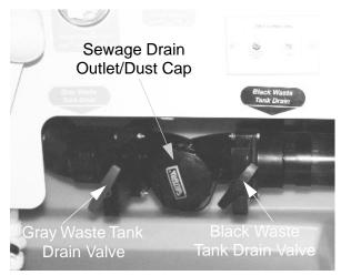
Holding Tank Drain Valves
