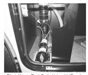
Black Waste Tank Drain Valve #1 (Front)
