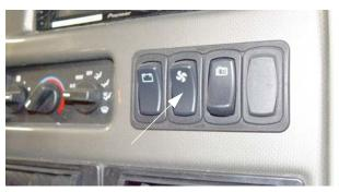
Defrost Fan Switch (Located on dash) -Typical View
