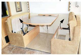
3. Release the lock rod on the bottom of the dinette table by pulling down.
