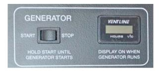
Refer to the hourmeter to determine when periodic maintenance is due and to record services which have been performed.
