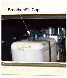
Hydraulic Oil Reservoir (Located behind driver side front tire)
