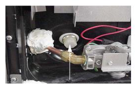
Water Heater Drain Plug (Remove with socket)
