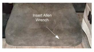
Remove the screws at the lower front corners on each side of the engine cover.
