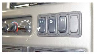
Battery Boost Switch (Located on dash) -Typical View
