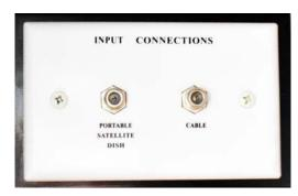
Satellite Dish and Cable TV Connections (Located in utility compartment, shoreline compartment, or water service center, depending on model)
