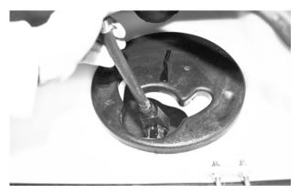
9. Then rotate to the smaller opening to enclose the cord.
