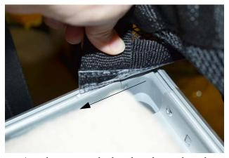
Attach straps to the brackets located on the cabinet face.
