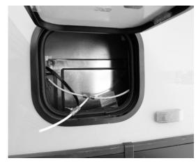
Ice Maker Drain Line (Located in exterior Residential Refrigerator service compartment)
