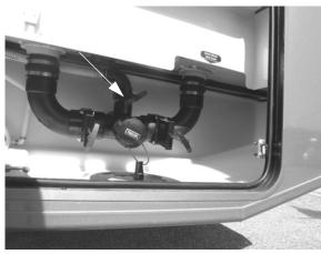
Black Waste Tank Drain Valve #2 (Front)
