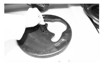
8. Rotate the cover to the largest hole to pass the cord end through.
