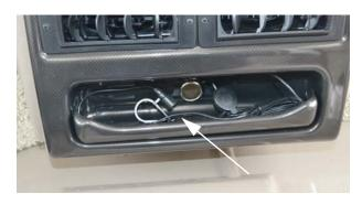
Bluetooth Microphone (Located on lower dash) -Typical View (if equipped)
