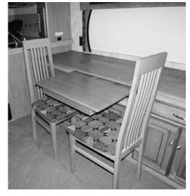
2. Bind chairs together with the provided strap, ensuring the strap goes through the ring located on the bottom side of the buffet table.
