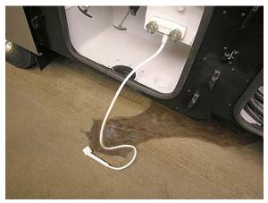
Using exterior shower to drain waterline
