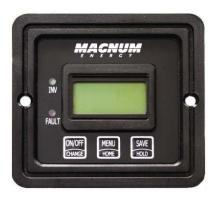
When the inverter is not being used, it should be shut off at the control panel. The inverter could drain the house batteries if the shoreline is not connected to external power and the House/ Coach Battery Disconnect switch is on.
